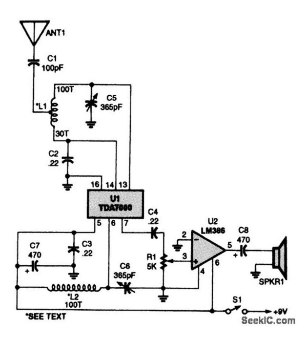
The schematic diagram of the receiver circuit is shown. About all you have to do is wind two coils, connect a few components together, and tie the input to a simple wire antenna, and a receiver is born. The two coils, L1 and L2, each comprised 100 turns of #28 enamel-covered copper magnet wire wound on T80-2 toroid cores (with a tap at the 30th turn on L1).
